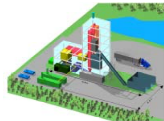
Figure 8: Design of a pre-commercial scale demonstration plant; capacity: 5.0 MW th fuel input (approx. 1000 kg dry /h), i.e. 1.5 MW el
