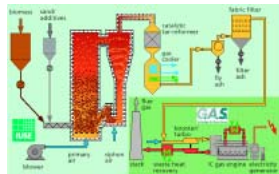
Figure 1: Process scheme: CFB gasifier with catalytic gas treatment and block heat & power plant (BHPP) with IC-engine
