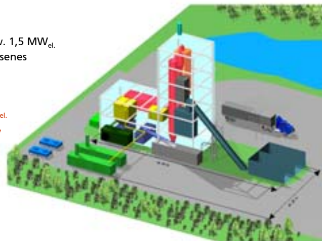
Design of a pre-commercial-scale demonstration plant; capacity: 5.0 MW fuel input or 1.5 MW el .
